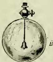
FIG. 2.—TRANSMISSION OF SOUND THROUGH A VACUUM.
